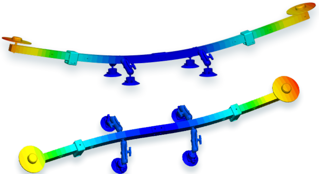
Eigenmode analysis of an ADAS Roof Mount Design by OxTS.
